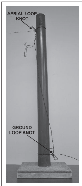
Figure 3-8. Method of tying wire lines at bottom and top support
